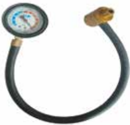
WESTINGHOUSE TEST ÜNİTESİ Vacuum Booster Test Unit
